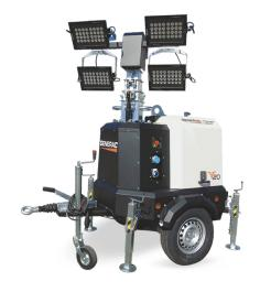
The V20 is a brand-new mobile light tower equipped with 4x320W high efficiency LED lamp floodlights. More than 160 hours of running time and one of the lowest sound pressure level in the industry: only 58 dB(A) at 7 meters.
