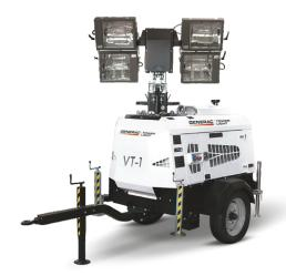
The first light tower in the world with integrated vertical telescopic mast. The VT1 has revolutionized the market for over fifteen years, becoming the best seller model of mobile light tower in Europe. Thanks to the 4x1000W powerful metal halide floodlights and the 8.5 meters mast, the VT1 can illuminate very big working areas.
